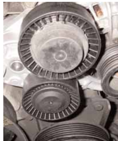
Photo #3 - New Tensioner And Idler
