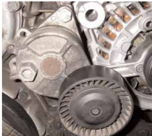
Photo #2 - Belt Tensioner Assembly
