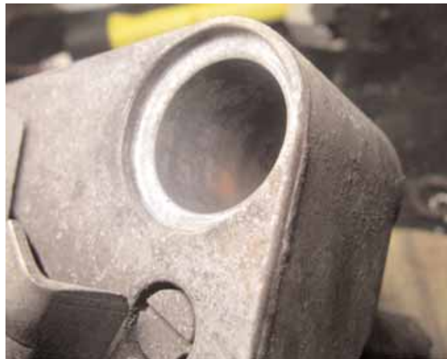
Photo #2 - Bore Ready For New Bushing
