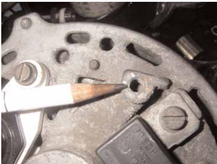
Photo #5 - Clean The Ground Connection
