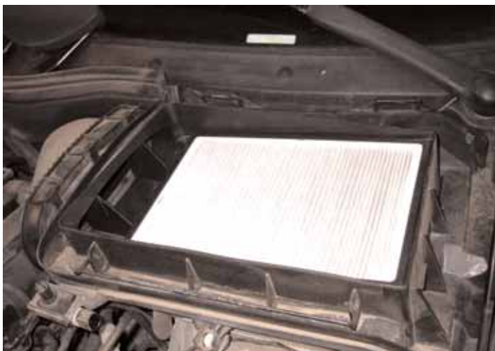
Photo #2 Cabin Filter Exposed
