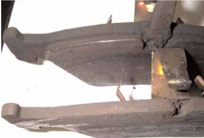
Photo #4 Worn E39 Front Brake Pads
