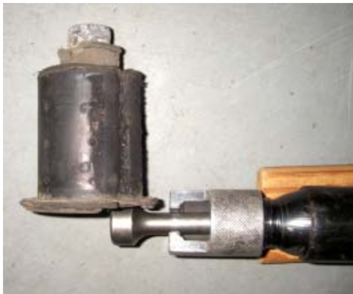
Photo #2 Bushing that "walked."
