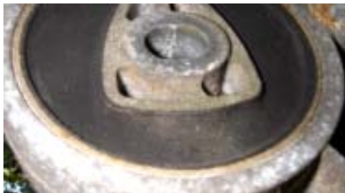
Photo #3 Good bushing
