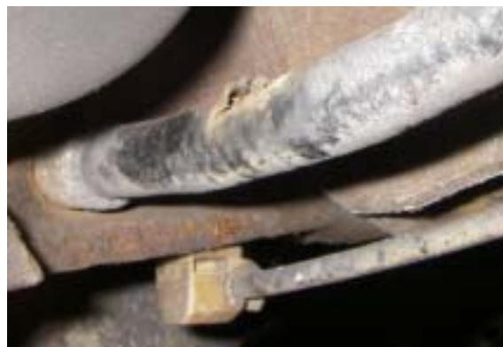
Photo #2 Parking Brake Cable
