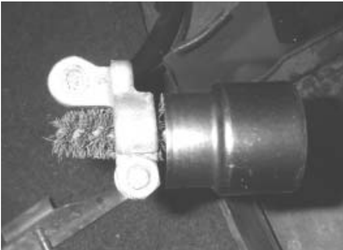
Photo #3 Wire brush to clean battery terminal cable.
