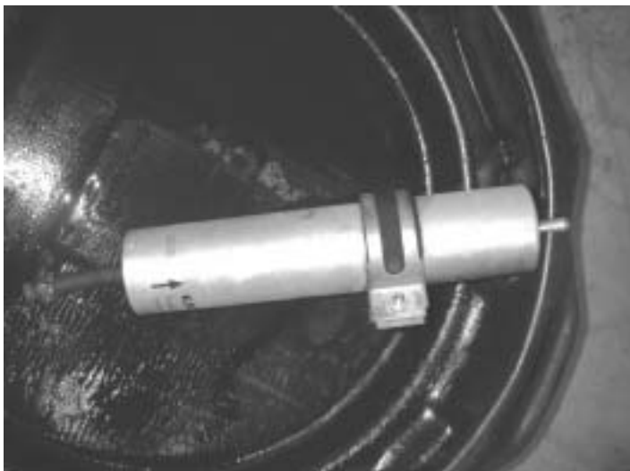
Photo #5 Inlet nipple plugged
