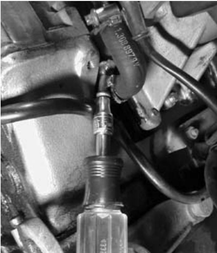
Photo #3 Using Socket To Change Hose Clamp
