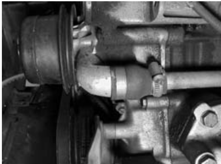
Photo #1 Heater Return Connection To Water Pump
