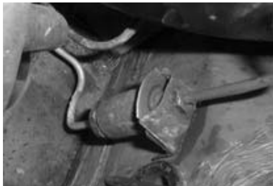
Photo #3 New Proportioning Valve
