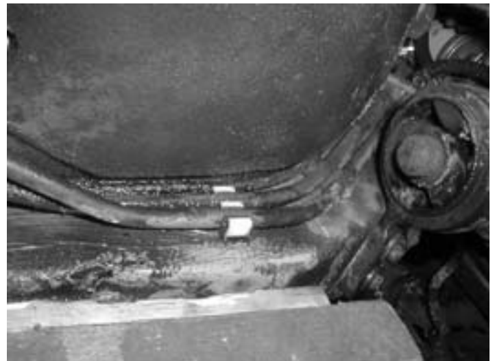
Photo #1 Burst Brake Line
