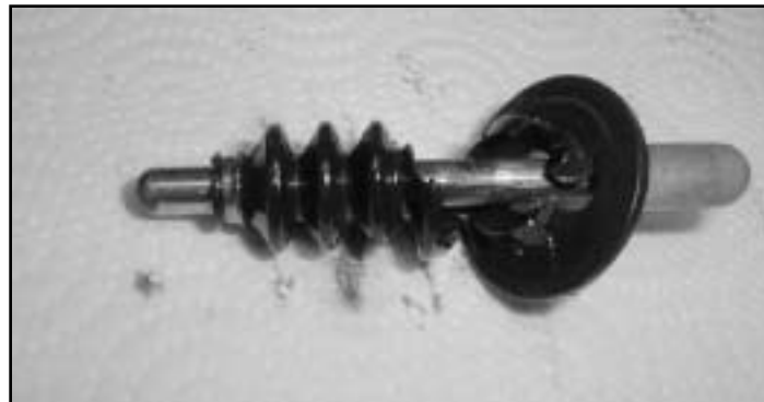
Photo 4: Slave cylinder pushrod and bellows
