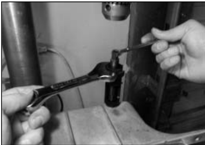
Photo 5: Installing the Heli-Coil with Special Tool
