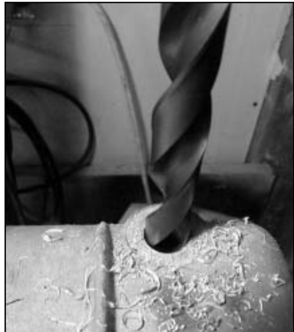
Photo 3: Drilling out the Damaged Threads
