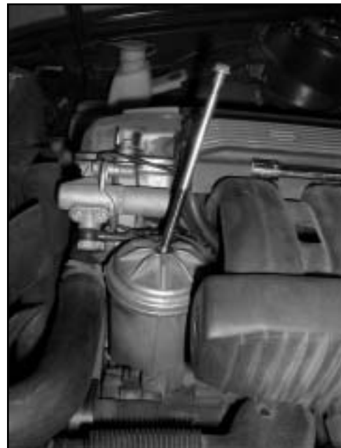
Photo 1: M50 Oil Filter Canister.
