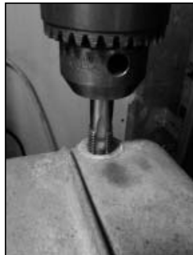
Photo 4: Preparing the Pan for the Helicoil
