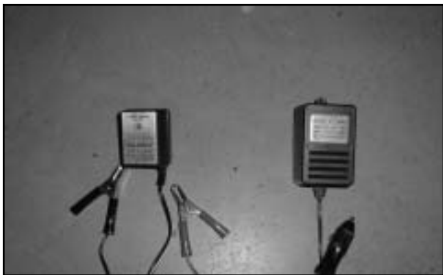
Photo 1: Battery Maintainers - One Modified With Cigar-Lighter Plug Photo: Philes Forum
