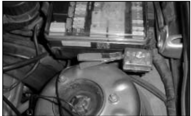
Photo 2: Maintainer Connections To Aux. Fuse Box In E30 M3 Photo: Philes Forum
