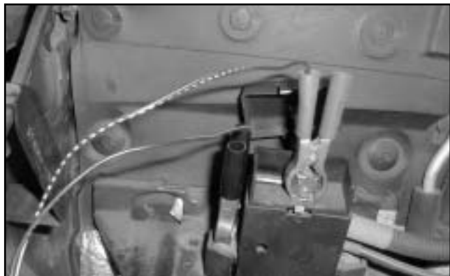
Photo 3: Maintainer Connections To Underhood Battery Junction In E36 325is Photo: Philes Forum
