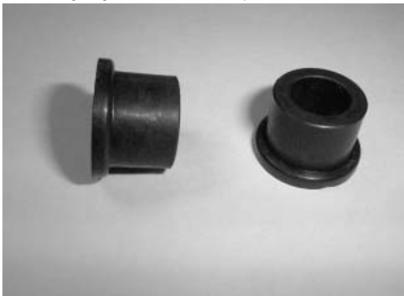
Photo 2: Alternator Bushings - Four Are Required
