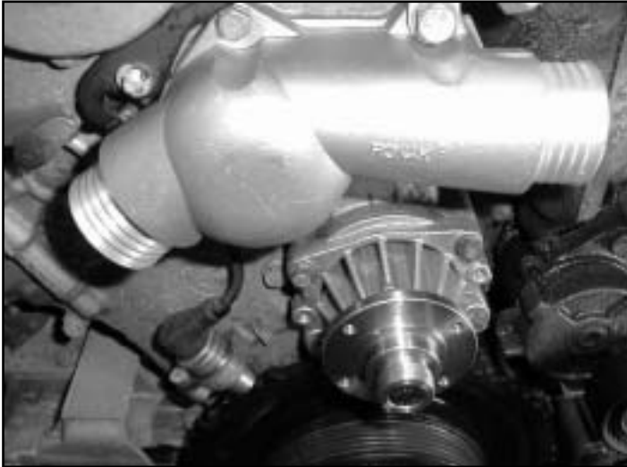
Photo 4: New Housing in Place.
