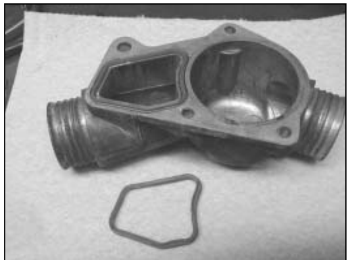
Photo 3: New Aluminum Housing and Profile Gasket
